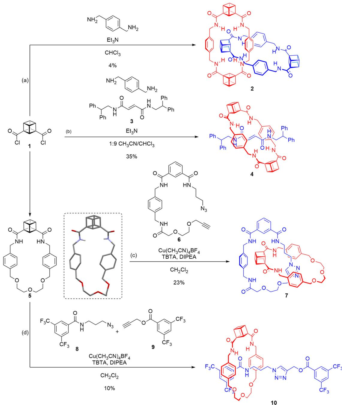
Scheme 1 Synthesis of cubane containing interlocked molecules. Inset: X-ray structure of macrocycle **5**.
