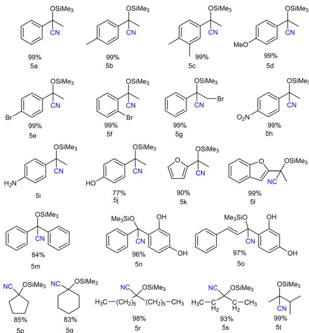
**Chart 1** Substrate scope for cyanosilylation of ketones using catalyst **3**. Reaction conditions: ketones (0.25 mmol), TMSCN (0.38 mmol, 1.5 equiv.), neat reaction at room temperature. The catalyst loading is 0.1 mol%. Reaction time: 15 min. Yield (%) determined by  $^1\text{H}$  NMR spectroscopy using mesitylene as an internal standard.
