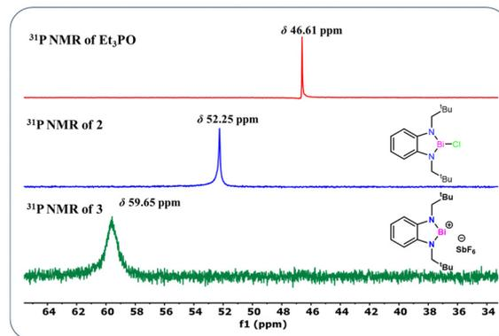
**Fig. 3** Stacked <sup>31</sup>P NMR spectra of **2–3** in the presence of Et<sub>3</sub>PO in CDCl<sub>3</sub> (Gutmann–Beckett method).
