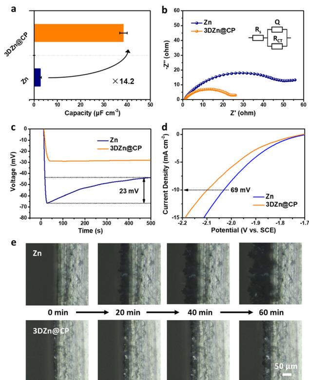
**Fig. 2** (a) The electrical double-layer capacitance analysis, (b) EIS plots, (c) voltage-time curves during Zn nucleation at  $1 \text{ mA cm}^{-2}$  and (d) hydrogen evolution linear polarization curves of commercial Zn and 3DZn@CP electrodes. (e) Cross-section OM images of the Zn and 3DZn@CP electrodes during Zn plating at  $20 \text{ mA cm}^{-2}$ .
