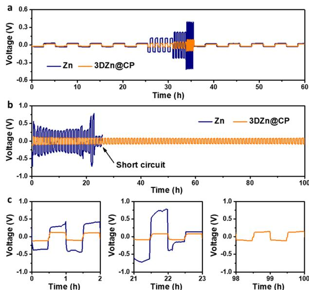
Fig. 3 (a) Rate performance of Zn||Zn and 3DZn@CP||3DZn@CP symmetrical cells at 1, 5, 10, 20  $\text{mA cm}^{-2}$  with a fixed areal capacity of  $2.5 \text{ mA h cm}^{-2}$ . (b) Voltage profiles and (c) enlarged voltage profiles of the specific cycles for Zn||Zn and 3DZn@CP||3DZn@CP symmetrical cells at  $20 \text{ mA cm}^{-2}$  and  $10 \text{ mA h cm}^{-2}$ .
