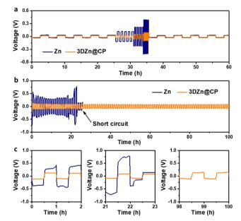
Fig. 3 (a) Rate performance of Zn||Zn and 3DZn@CP||3DZn@CP symmetrical cells at 1, 5, 10, 20 mA cm<sup>-2</sup> with a fixed areal capacity of  $2.5 \text{ mA h cm}^{-2}$ . (b) Voltage profiles and (c) enlarged voltage profiles of the specific cycles for Zn||Zn and 3DZn@CP||3DZn@CP symmetrical cells at  $20 \text{ mA cm}^{-2} \text{ and } 10 \text{ mA h cm}^{-2}$
