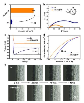
Fig. 2 (a) The electrical double-layer capacitance analysis, (b) EIS plots, (c) voltage—time curves during Zn nucleation at 1 mA cm $^{-2}$  and (d) hydrogen evolution linear polarization curves of commercial Zn and 3DZn@CP electrodes. (e) Cross-section OM images of the Zn and 3DZn@CP electrodes during Zn plating at 20 mA cm $^{-2}$ .
