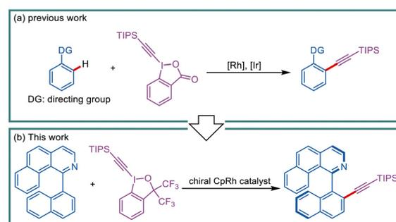
Scheme 1 Transition-metal-catalyzed C–H alkylation reactions with EBX reagents.
