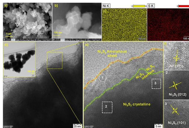
Fig. 3 (a) and (b) FESEM images, (c) elemental mapping, (d) TEM and (e) HR-TEM images showing lattice fringes of NNS/NNS<sub>x</sub>.
