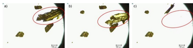
Fig. 5 Still images taken from a video recorded of AnThio during a variable-temperature experiment on a microscope (Video S2, ESI†). AnThio crystals are recrystallized material (a) before, (b) during, and (c) after thermosalience. Scale bars are 150 μm.
