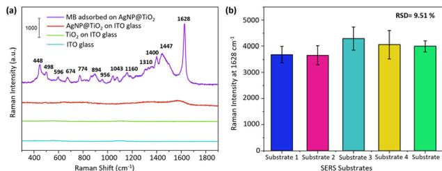
**Fig. 3** (a) Raman spectrum of different chip layers: ITO glass (cyan), TiO<sub>2</sub> film (green), background spectrum of silver nanoparticles at TiO<sub>2</sub> (red), and SERS spectrum of 10 μM methylene blue adsorbed on the surface of the complete SERS substrate (purple). (b) Substrate-to-substrate variation for five SERS substrates. The peak at 1628 cm<sup>-1</sup> in the SERS spectrum was used to calculate the mean intensity ( $N = 5$ ).
