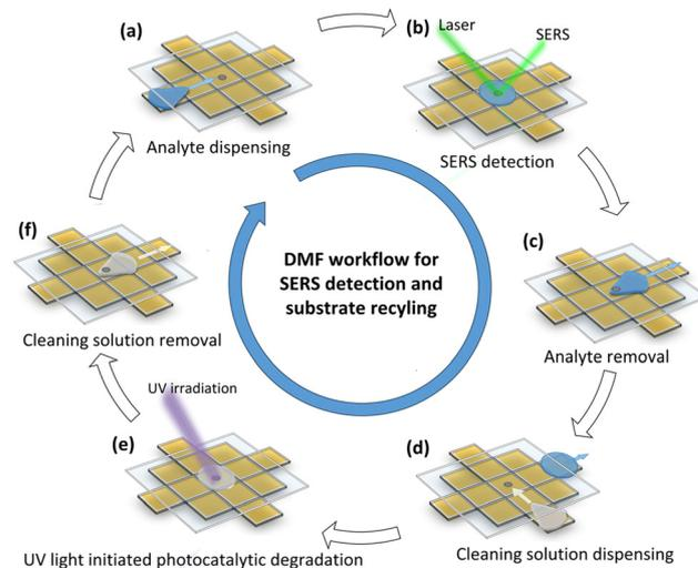
**Fig. 4** (a–f) Schematic for the droplet actuation steps inside DMF integrated AgNP@TiO<sub>2</sub> SERS substrate for consecutive detection and recycling process. The blue arrow (inside chip) indicates the MB droplet actuation direction; the white arrow (inside chip) indicates the cleaning solution droplet actuation direction.
