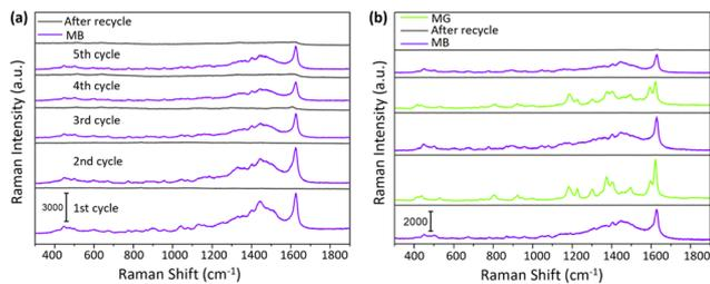
**Fig. 6** (a) SERS spectra of MB (10  $\mu\text{M}$ ) adsorbed onto the DMF integrated AgNP@TiO<sub>2</sub> SERS substrate showing five “detection-recycling” cycles. (b) SERS spectra of MB and MG (10  $\mu\text{M}$ ) on the SERS substrate in alternating detection processes before and after recycling.
