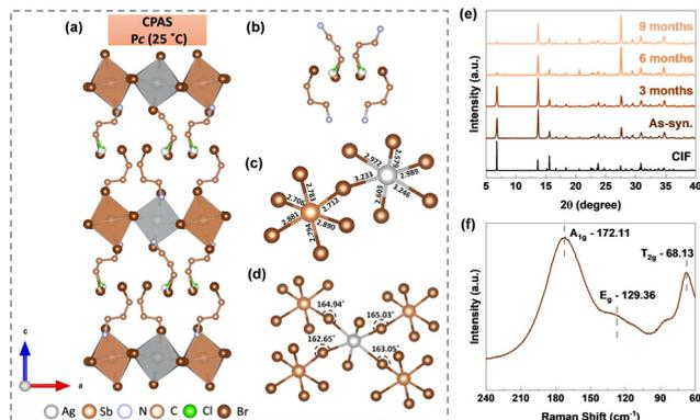
**Fig. 1** Structural properties of CPAS. (a) Single crystal X-ray structure of  $\text{Cl}_{0.26}\text{Br}_{3.74}\text{PA}_4\text{AgSbBr}_8$  at 25 °C. Hydrogen atoms are omitted for clarity. (b) Zoomed-in image of the halogen ( $\text{Cl}^-/\text{Br}^-$ ) distribution in the organic spacer. (c) and (d) Octahedral bond length and angle arrangements. (e) Powder XRD comparison between simulated and as-synthesized materials and stability over nine months. (f) Raman spectra.
