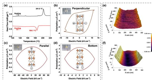
**Fig. 2** (a) Differential scanning calorimetric measurement. (b)–(d) *P–E* hysteresis loop studies carried out in perpendicular, parallel and bottom configurations for CPAS single crystals. Insets represent crystal arrangements and optical images of the device. (e) AFM topography image and (f) PFM image of the CPAS single crystal at an applied tip voltage of 5 V. The colour scale is given on the far right.
