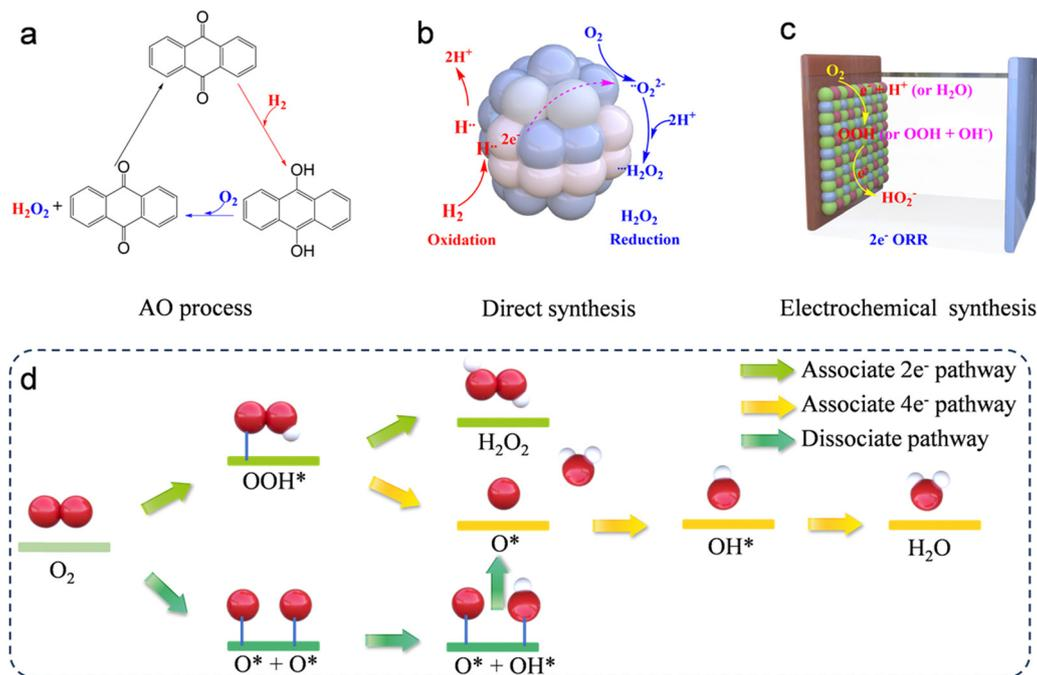
Fig. 1 Illustration of hydrogen peroxide production via (a) traditional anthraquinone process, (b) the direct synthesis, and (c) electrochemical two-electron oxygen reduction reaction. (d) Illustration of the proposed ORR process.
