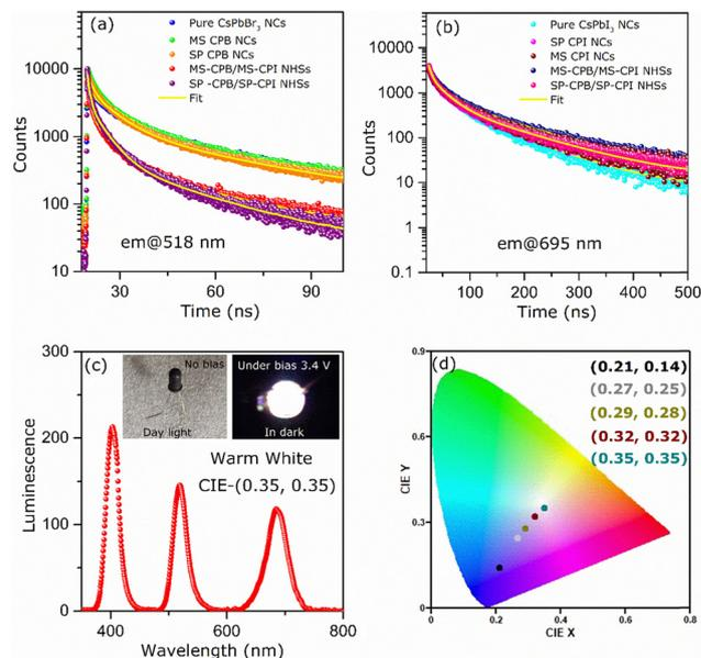
**Fig. 3** TRPL decay curves of (a) pristine CPB, SP/MS-CPB, and their corresponding NHSSs; (b) pristine CPI, SP/MS-CPI, and their corresponding NHSSs; (c) PL spectra of pc-LED fabricated by stacking SP-CPB and SP-CPI on 405 nm emitting commercial LED. Inset shows photographs of the LED without and with applied bias of 3.4 V; (d) CIE plot for LEDs fabricated with different proportions of SP-CPB:SP-CPI.
