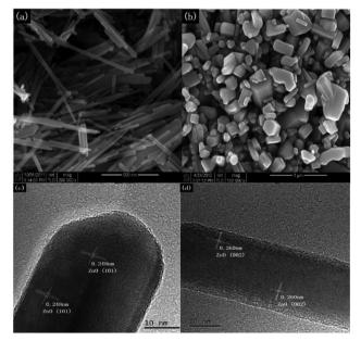
Fig. 13 (Top) SEM imaging of (a) 1D-nanorod ZnO and (b) bulk ZnO. (Bottom) TEM imaging of the obtained nanorods. Credit: Z. R. Tang, X. Yin, Y. Zhang and Y. J. Xu, RSC Adv., 2013, 3, 5956-5965.
