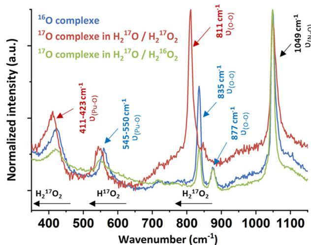
Fig. 3 Raman spectra of the green peroxo compound of Pu(IV) (nitric system) prepared in H<sub>2</sub><sup>16</sup>O/H<sub>2</sub><sup>16</sup>O<sub>2</sub> (blue spectrum), H<sub>2</sub><sup>17</sup>O/H<sub>2</sub><sup>17</sup>O<sub>2</sub> (red spectrum) and H<sub>2</sub><sup>17</sup>O/H<sub>2</sub><sup>16</sup>O<sub>2</sub> (green spectrum).
