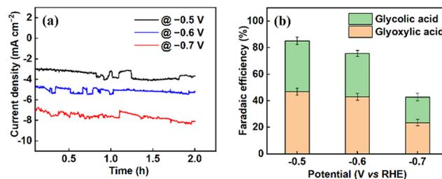
**Fig. 2** (a) The current densities of titanium electrodes at three different applied potentials (-0.5 V, -0.6 V and -0.7 V vs. RHE) and (b) the average faradaic efficiency for production of glyoxylic and glycolic acids during bulk electrolysis of 0.03 M oxalic acid for 2 hours, using Ti foil as a working electrode and Pt foil as a counter electrode in an H-cell at 25 °C.
