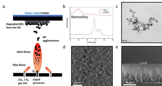
**Fig. 1** (a) Scheme of the FSP process with nanoparticles deposited on substrates by thermophoresis. (b) X-ray diffractogram of the 50 at% AgAu/SiO<sub>2</sub> nanoalloy in powder form (black line) and as-deposited on the Si substrate (red line). (c) Transmission electron microscopy (TEM) image showing the alloyed nanoaggregates. (d) SEM image of the homogeneous coating surface from the top and (e) side.
