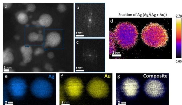
**Fig. 2** (a) High resolution TEM image of the alloyed NPs with the respective crystal phases (b) and (c). (d) Ag rich "shells" in the alloy composition. (e)–(g) Elemental mapping of Ag, Au in separate images and as a composite.
