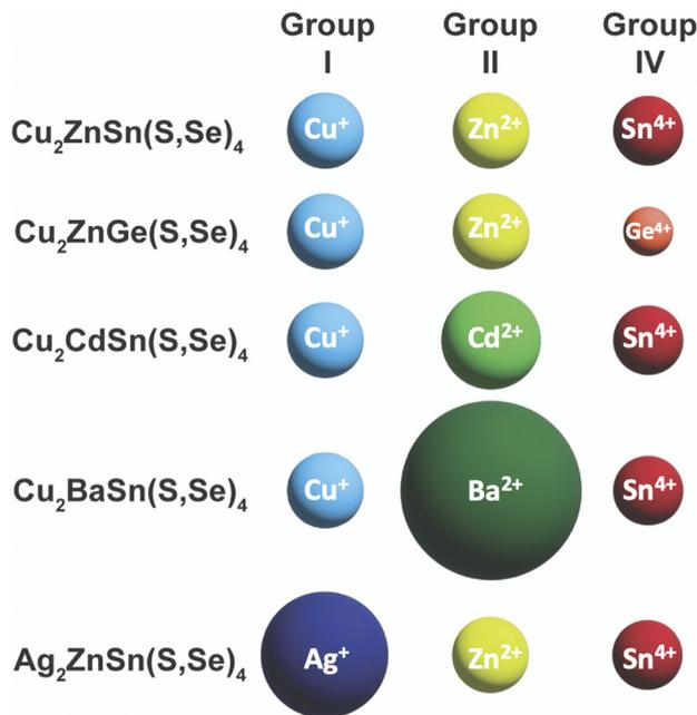
Fig. 9 Comparison of ionic radii of cations in  $\text{Cu}_2\text{ZnSn}(\text{S,Se})_4$  and substituted variants. Ionic radii are based on a coordination number of 4, except for  $\text{Ba}^{2+}$  with a coordination number of 8:  $\text{Cu}^+$  – 0.6 Å,  $\text{Ag}^+$  – 1 Å,  $\text{Zn}^{2+}$  – 0.6 Å,  $\text{Cd}^{2+}$  – 0.78 Å,  $\text{Ba}^{2+}$  – 1.42 Å,  $\text{Sn}^{4+}$  – 0.55 Å,  $\text{Ge}^{4+}$  – 0.39 Å.<sup>117</sup>
