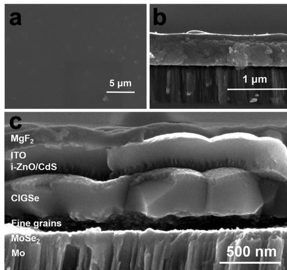
Fig. 5 (a) Top view and (b) side view SEM images of nanoparticulate  $\text{Cu}(\text{In,Ga})(\text{S,Se})_2$  precursor film and (c) side view SEM image of coarsened  $\text{Cu}(\text{In,Ga})(\text{S,Se})_2$  absorber in a completed device. Reprinted with permission.<sup>36</sup> Copyright 2016 Royal Society of Chemistry.
