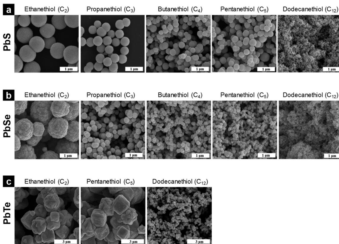
Fig. 14 SEM images showing the morphological control *via* thiol selection in the synthesis of (a) PbS, (b) PbSe, and (c) PbTe particles. Reprinted with permission.<sup>199</sup> Copyright 2019 American Chemical Society.
