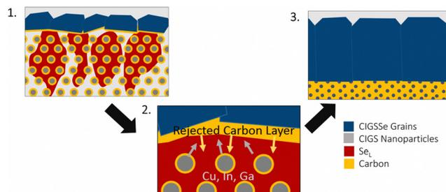
Fig. 6 Schematic of grain growth mechanism and fine-grain layer formation via liquid selenium flux mechanism. Reprinted with permission.<sup>78</sup> Copyright 2019 Elsevier.
