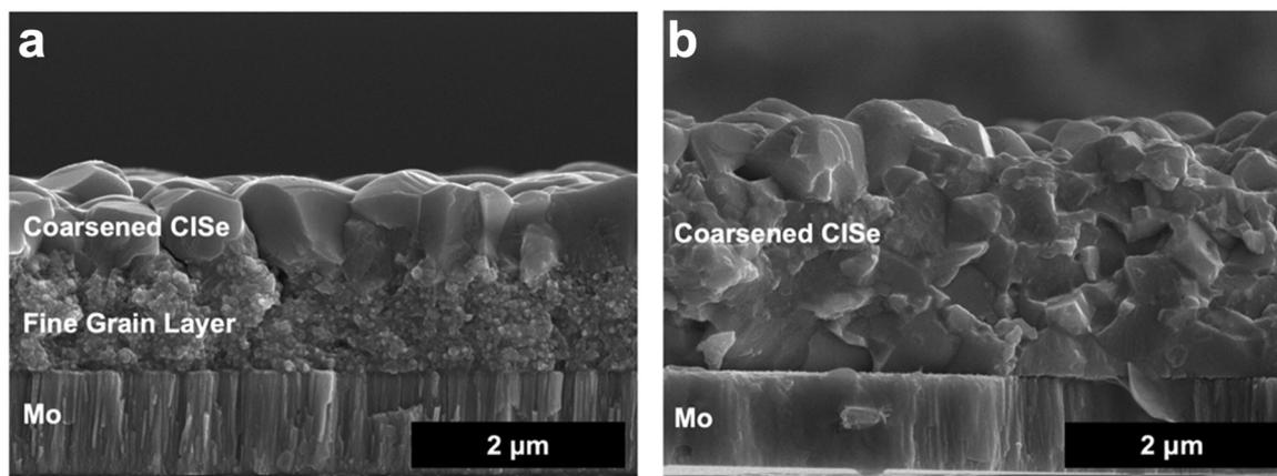
Fig. 7 (a) SEM of coarsened CuInSe<sub>2</sub> film made from a thick CuInS<sub>2</sub> precursor film showing a large fine grain layer and (b) SEM of coarsened CuInSe<sub>2</sub> film made from a thick CuInSe<sub>2</sub> precursor film with no fine grain layer. Reprinted with permission.<sup>79</sup> Copyright 2023 American Chemical Society.
