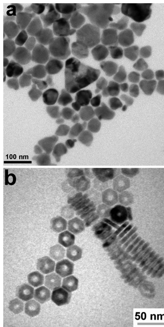
Fig. 3 (a) Nanoparticles and (b) nanorings of CuInSe<sub>2</sub> with morphology controlled by reaction conditions. Reprinted with permission.<sup>56</sup> Copyright 2008 American Chemical Society.
