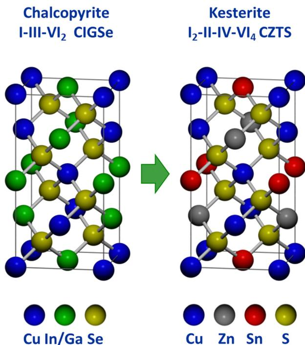
Fig. 8 Comparison of chalcopyrite and kesterite crystal structures.<sup>93</sup>
