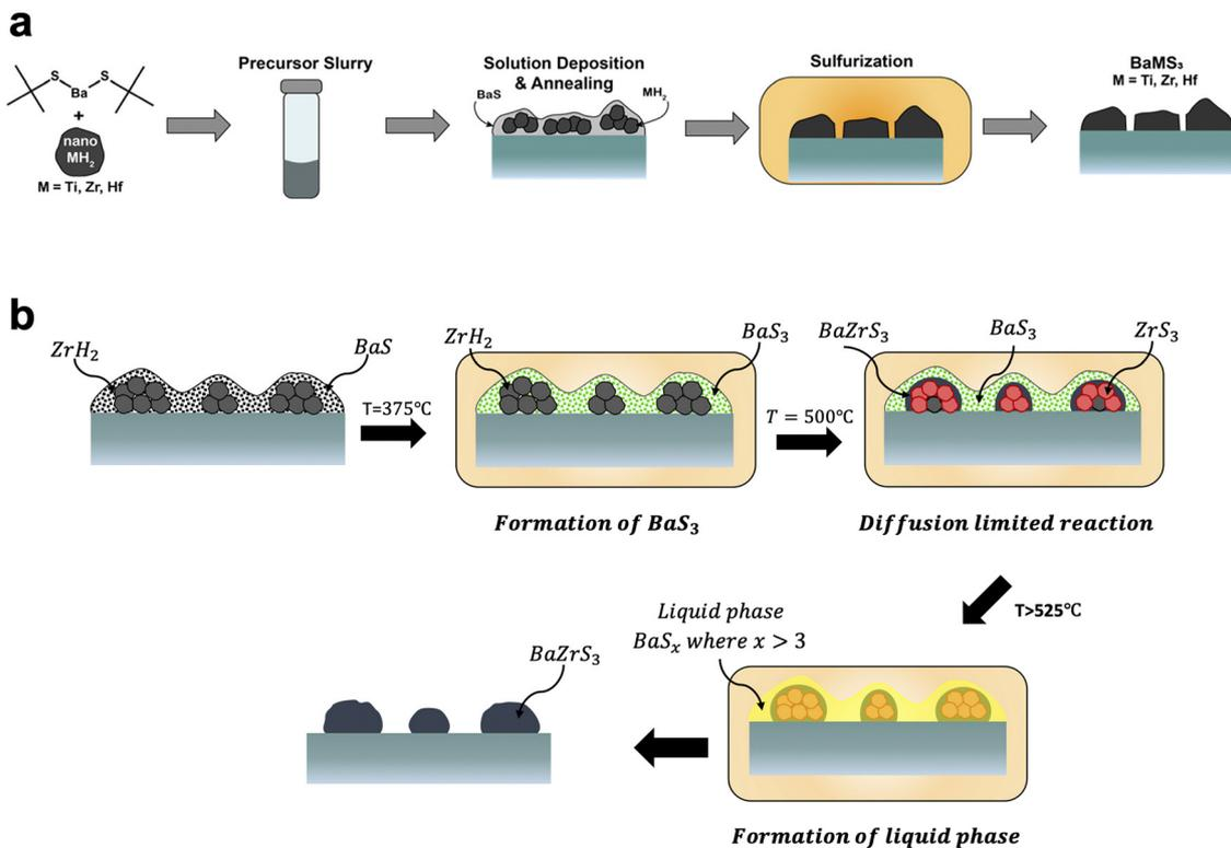
Fig. 10 (a) Schematic of solution deposition approach for the synthesis of  $\text{BaMS}_3$  ( $M = \text{Ti, Zr, Hf}$ ) materials. Reprinted with permission.<sup>177</sup> Copyright 2022 American Chemical Society. (b) Schematic of the barium polysulfide liquid-flux assisted formation of  $\text{BaZrS}_3$ . Adapted with permission.<sup>178</sup> Copyright 2023 Wiley-VCH.
