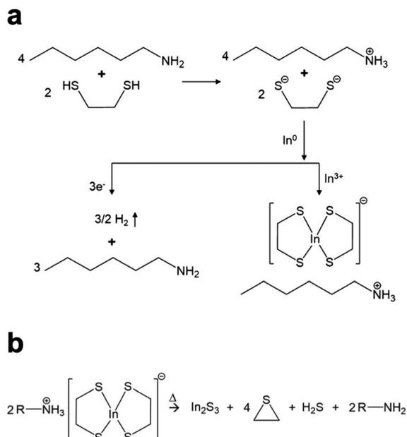
Fig. 2 (a) Reactive dissolution mechanism for amine–thiol reaction with indium metal. Reprinted with permission.<sup>28</sup> Copyright 2019 American Chemical Society. (b) Decomposition mechanism of the resulting indium thiolate into indium sulfide. Reprinted with permission.<sup>32</sup> Copyright 2019 American Chemical Society.
