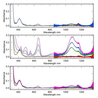
Fig. 1 Time-dependent UV-Vis-NIR spectra of 10 mM uranyl(v) mixtures with 90.4 mM Gly (top), Val (middle), and Phe (bottom) under illumination of 365 nm light. Before illumination (black), 60 s (red), 360 s (green), 600 s (blue), and 900 s (pink) after illumination.
