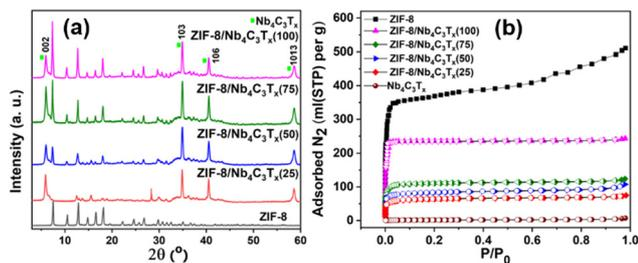
Fig. 2 (a) XRD pattern of various ZIF-8/ $\text{Nb}_4\text{C}_3\text{T}_x$  composites. (b)  $\text{N}_2$  adsorption isotherms of ZIF-8,  $\text{Nb}_4\text{C}_3\text{T}_x$  and their composites (the closed symbols represent adsorption, while the open symbols represent desorption).
