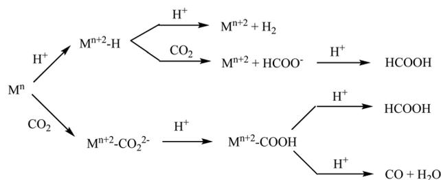
**Scheme 1** Selectivity for 2e<sup>−</sup>/2H<sup>+</sup> reduction of CO<sub>2</sub> via the M–COOH pathway.
