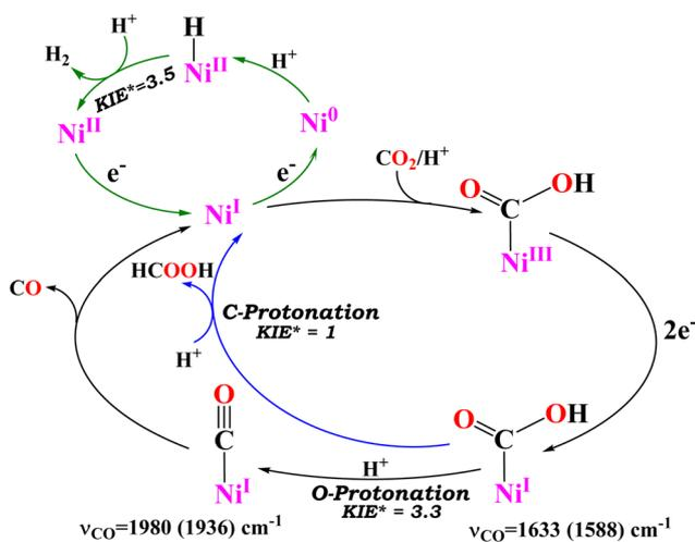
**Scheme 2** Reaction mechanism of different pathways of  $\text{CO}_2/\text{CO}$  (black arrow) and  $\text{CO}_2/\text{HCOOH}$  (blue arrow) along with the HER (green arrow). The relative KIE ( $\text{KIE}^*$ ) is shown for all the reaction pathways.
