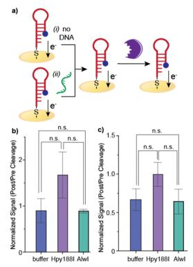
Fig. 3 Non-hybridization conditions. (a) Addition (i) buffer or (ii) noncomplementary DNA does not impact hairpin. Signal change is not significant for buffer only (b) or non-complementary DNA (c). Error bars represent standard error (n = 7).
