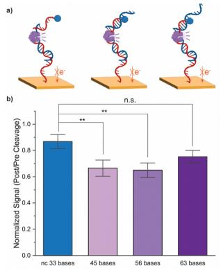
Fig. 4 Influence of target sequence length on assay efficacy. (a) Three complementary sequences of increasing length, ranging from 45 bases to 63 bases, and one non-complementary sequence of 33 bases were tested, (b) MB signal decreases after hybridized DNA is treated with 100 U mL<sup>-1</sup> of Hpy1881. There is statistically significant decrease in the MB signal for target lengths of 45 bases and 56 bases. Error bars represent standard error (n = 15).
