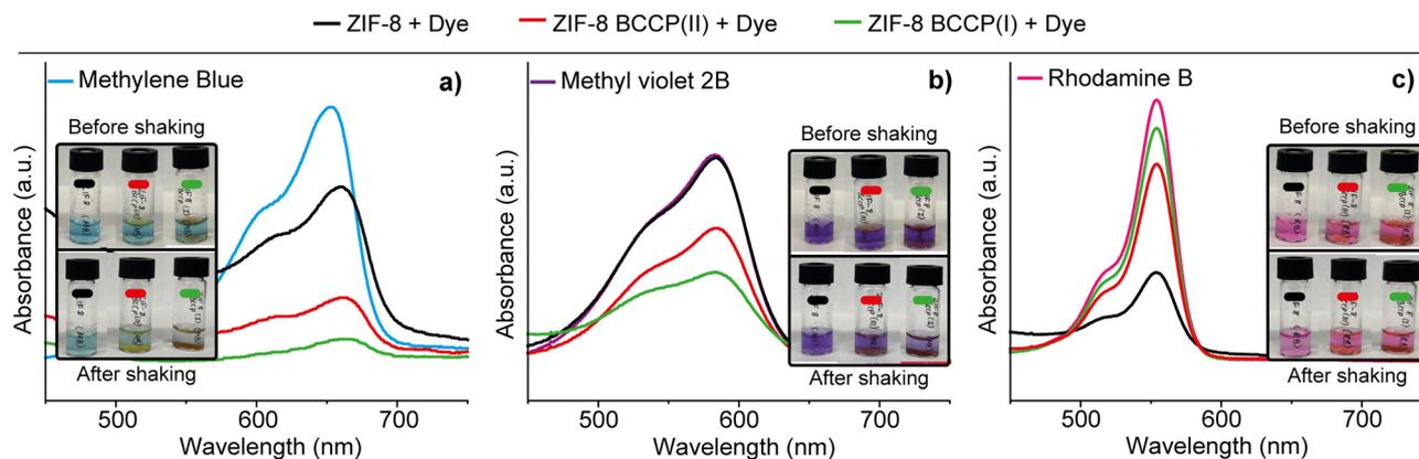
Fig. 4 Absorption spectra of organic micropollutants: (a) methylene blue, (b) methyl violet 2B, and (c) rhodamine B before and after treatment with ZIF-8 structures. The insets show the aqueous solutions of dyes before (top layers) and after shaking (bottom layers) with ZIF-8 structures for 2 hours: (left) methylene blue, (middle) methyl violet 2B, and (right) rhodamine B.
