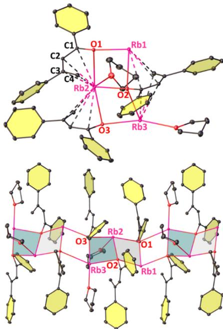
Fig. 3 (top) Asymmetric unit of the structure of  $[(\text{RbOC}(\text{Ph})=\text{C}(\text{H})\text{C}(\text{Ph})=\text{CH}_2)_3 \cdot (\text{THF})_2]_\infty$  (**2-Rb**); (bottom) section of the infinite ladder of **2-Rb**. For clarity, thermal ellipsoids displayed at 20% probability, H atoms omitted, and aromatic rings shaded yellow.  $\text{Rb}_2\text{O}_2$  rings are shaded to display the ladder's linear growth.
