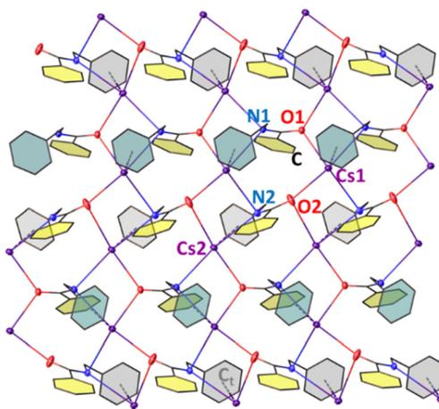
Fig. 5 Section of the network structure of  $[\text{CsOC}(\text{Ph})=\text{NCH}_2\text{Ph}]_\infty$  (**3-Cs**). Thermal ellipsoids of all non-C/H atoms displayed at 25% probability, and C atoms reduced to 5% for clarity. H atoms omitted, and aromatic rings shaded in yellow, grey, and teal for clear depiction of  $\text{M} \cdots \pi$  interactions.  $\text{C}_t$  depicts centroid of Ph rings.
