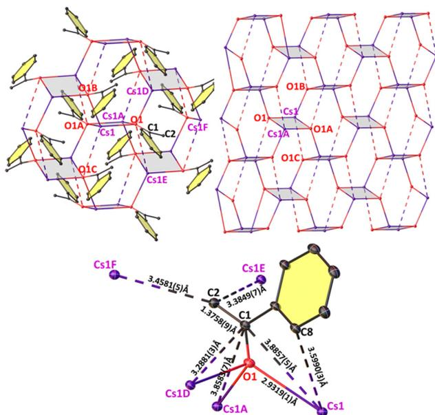
Fig. 2 (top left) Section of the infinite network structure of  $[\text{CsOC}(\text{Ph})=\text{CH}_2]_\infty$  (**1-Cs**); (top right); section displaying the fused distorted hexagonal Cs–O prisms. All C atoms omitted for better visualization; (bottom) section describing the interaction of five Cs atoms with one enolate anion. For clarity, thermal ellipsoids displayed at 20% probability, H atoms omitted, and aromatic rings shaded yellow.
