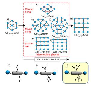
Fig. 1 (b)-(f) Selected intermediate phases at the transition between (a) triangular and (g) square LC honeycombs; the shown nets represent cuts through the honeycombs perpendicular to the c-axis (see Fig. 3c.i for spatial models), the rod-like cores are organized along the dark lines and the blue dots represent the polar columns of the end groups, the side chains fill the cells: (h) and (i) bolapolyphiles forming these tiling patterns and (i) compounds under discussion herein.
