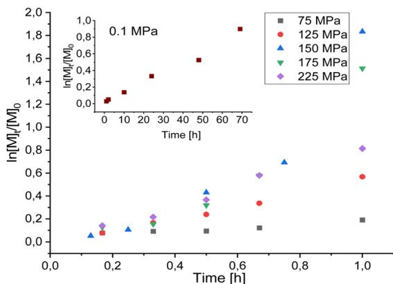
Fig. 1 The semilogarithmic kinetic plots as a function of time for HP&LI ATRP of OEOMA<sub>500</sub> under different pressures.
