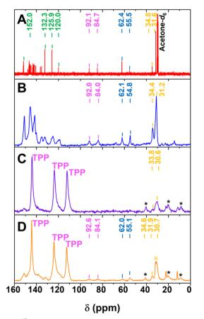
Fig. 3 The  $^{13}\text{C}$  NMR spectra of  $\boldsymbol{1}$  in a CS $_2$  solution with the internal standard of acetone- $d_6$  at 25 °C (A), of **1** in solid state (B), and the solidstate  $^{13}$ C CP MAS NMR spectra of 5%**1**@TPP- $d_{12}$  (C) and 10%**1**@TPP- $d_{12}$  (D). The black asterisks indicate spinning sidebands
