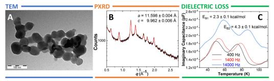
Fig. 2 A TEM visualization of  $10\%1_0$ TPP- $d_{12}$  (A). PXRD pattern of  $10\%1_0$ TPP- $d_{12}$ . The black line represents the diffraction data, while the red curve reflects the fit (B). The dielectric loss of 10%1@TPP-d<sub>12</sub> recorded between 20 and 110 K. Black – 400 Hz, red – 1400 Hz, and blue – 14000 Hz (C).
