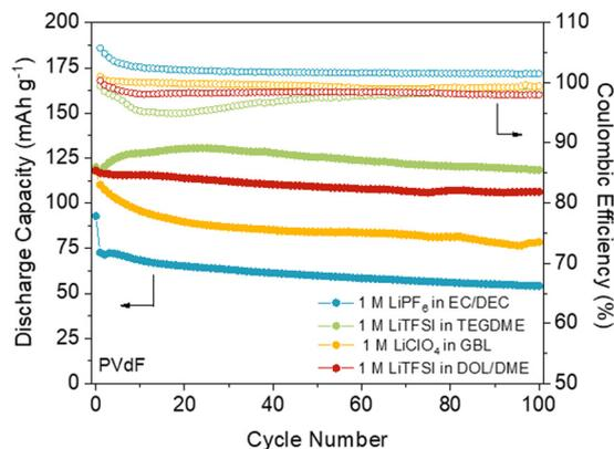
Fig. 8 DAAQ-TFP-COF electrode performance with PVdF as a binder at 150 mA g<sup>-1</sup> (1C) in four different electrolytes: 1 M LiTFSI in DOL/DME (1:1, vol%) (red), 1 M LiTFSI in TEGDME (green), 1 M LiPF<sub>6</sub> in EC/DEC (1:1, vol%) (blue), and 1 M LiClO<sub>4</sub> in GBL (yellow). Adapted with permission from ref. 85.
