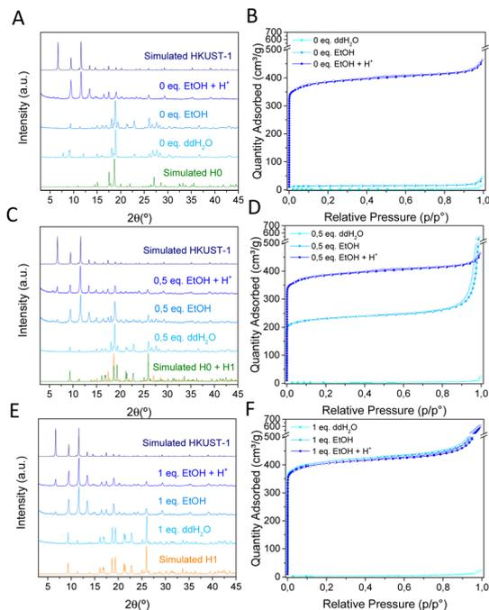
Fig. 1 XRPD patterns (left) and  $N_2$  sorption isotherms (right) of Cu-BTC materials synthesized with (A, B) 0 equivalents, (C, D) 0.5 equivalents and (E, F) 1 equivalent of HCl and the corresponding products washed with water ( $ddH_2O$ ), ethanol (EtOH) or ethanol and acid (EtOH +  $H^+$ ). H0: CCDC 609754,<sup>11</sup> H1: CCDC 1288676.<sup>12</sup>
