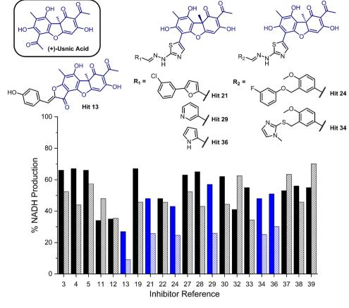
Fig. 2 Bar chart comparing percentage NADH production in the presence of each of 21 potential inhibitors without preincubation with GMD (solid bars) and with preincubation for 1 hour with GMD (hashed bars). Complete structure panel is shown in the ESI,† Section S1.2. The 6 best performing compounds are highlighted blue. Percentage NADH production was determined relative to a positive control containing no inhibitor and 1.
