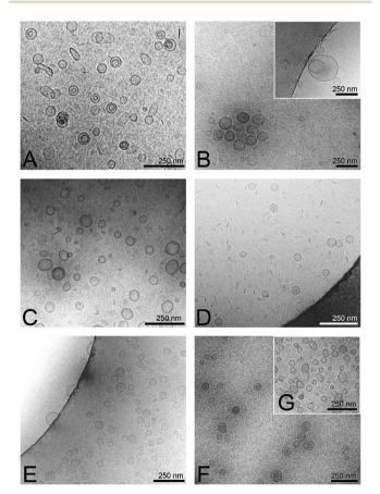
Fig. 2 Cryo-TEM images of hybrid-vesicles with a scale bar of 250 nm. (A) (EO) $_3P_{26}A$ \_Hy\_20 mol%, (B) (EO) $_3P_{11}A$ \_Gl\_5%, (C) (EO) $_3P_{42}A$ \_Gl\_5%, (D) (EO) $_3P_{42}A$ \_Gl\_20%, (E) (EO) $_2P_{48}A$ \_Co\_10%, (F) (EO) $_3P_{18}A$ \_Co\_10% and (G) (EO) $_3P_{52}A$ \_Co\_10% polymers embedded in POPC lipid.
