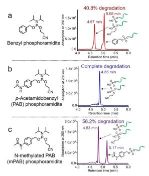
Fig. 2 HPLC traces of (a) DNA-benzyl conjugate (ODN1), (b) DNA-PAB conjugate (ODN2) and (c) DNA-mPAB conjugate (ODN3) after deprotection by aqueous ammonia at room temperature for two hours. The percentages of degradation of ODN1, ODN2 and ODN3 are 40.8%, almost 100% and 56.2%, respectively, demonstrating that N-methylation of the PAB-phosphodiester enhances its stability during oligonucleotide synthesis and deprotection.
