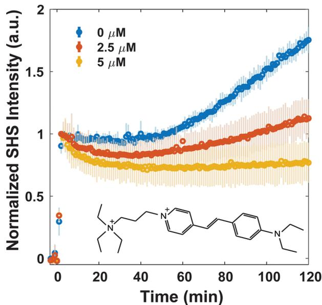
Fig. 3 Normalized trSHS trials of 16  $\mu\text{M}$  FM 2-10 with *S. aureus* with increasing concentrations of MLT. The structure of FM 2-10 is shown in the plot. For each concentration of MLT,  $n = 3$ . Averaged data is shown as circles and the shaded error bars represent the standard deviation between the individual normalized trials.
