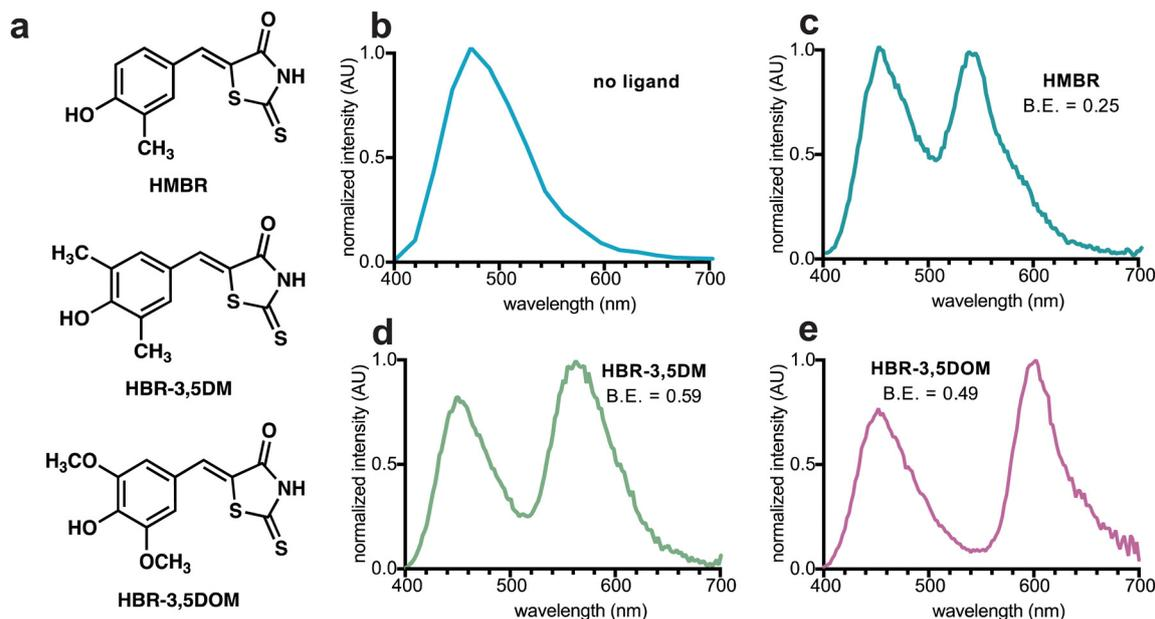
Fig. 2 Bioluminescence emission spectra with BREAKFAST probes. (a) Structures of candidate fluorogens. Spectra were acquired with BREAKFAST in the presence of (b) Fz only, (c) Fz and **HMBR**, (d) Fz and **HBR-3,5DM** or (e) Fz and **HBR-3,5DOM**. For all measurements, Fz and fluorogen were used at equimolar ratios (50  $\mu\text{M}$  or 1 : 50 dilution of commercial stocks). B.E. = BRET efficiency.
