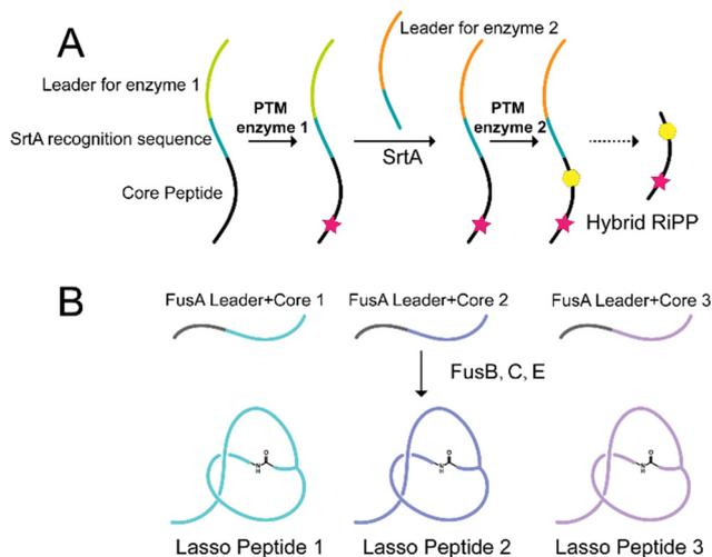
**Fig. 7** Well-designed RiPPs engineering systems. (A) A schematic representation of the leader peptide exchange strategy. Sortase A can exchange the leader peptides for one core peptides, thus enabling modifications with different PTM enzymes. (B) A schematic representation of the chimeric substrate strategy. Different core peptides are fused to the same FusA leader peptide, and FusB, C, and E can recognize them, respectively, leading to the production of different lasso peptides.
