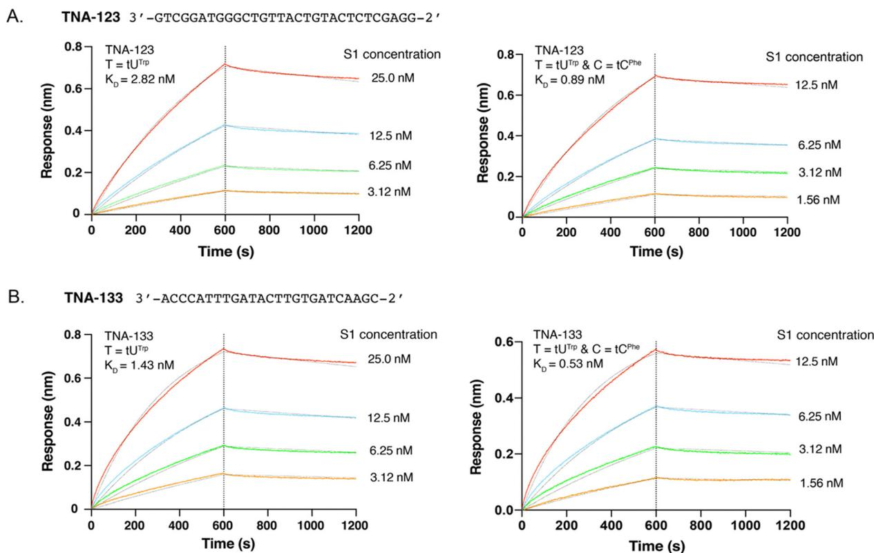
Fig. 3 Background-subtracted BLI sensorgrams comparing the binding kinetics to S1 of two aptamers containing either a single modification (tU<sup>Trp</sup>) or a doubly modified sequence (tU<sup>Trp</sup> and tC<sup>Phe</sup>). (A) BLI sensorgrams for aptamer TNA-123. (B) BLI sensorgrams for aptamer TNA-133. Aptamers were enzymatically prepared using a 5' DNA primer (not shown).
