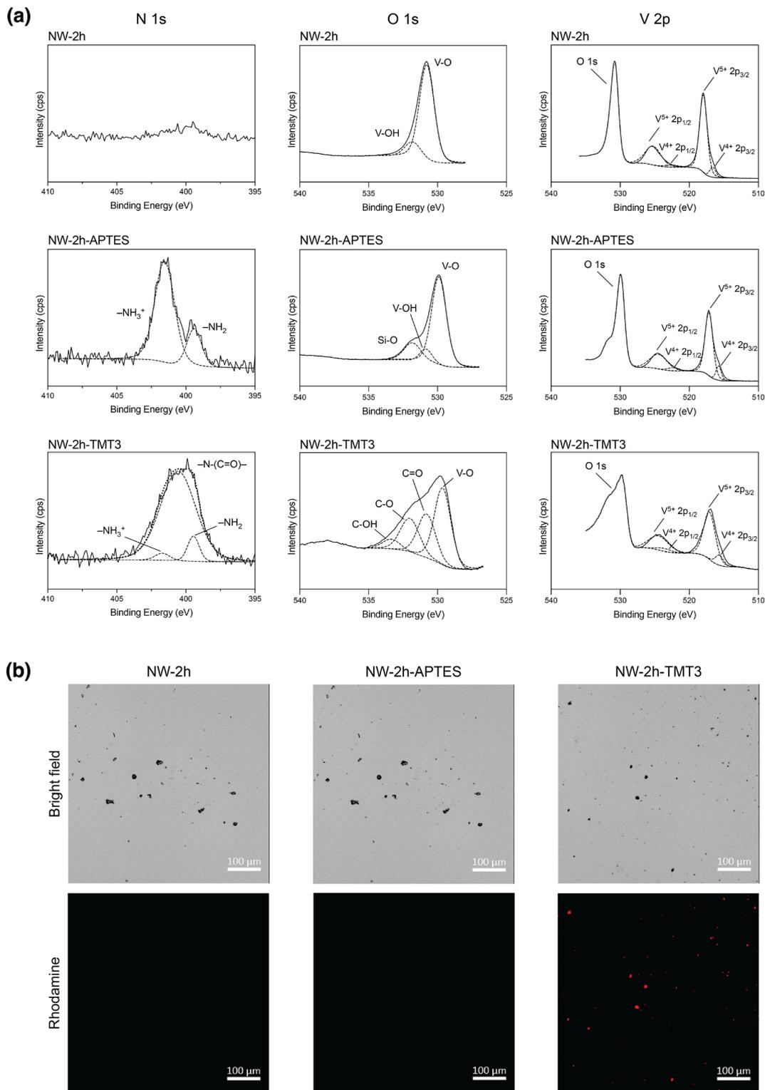
**Fig. 2** Surface modification of NW-2 h with trans-tympanic peptides. (a) High-resolution X-ray photoelectron spectroscopy (XPS) scan on N (1s), O (1s), and V (2p) showing changes to the surface binding energy on NW-2 h before and after APTES and TMT3 coating. (b) Representative confocal microscopy images showing large clusters of NW-2 h, NW-2 h-APTES and NW-2 h-TMT3; fluorescent signals from the rhodamine tag on TMT3 was only witnessed from NW-2 h-TMT3.
