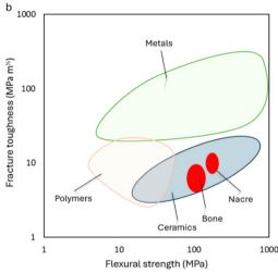
Fig. 5 Exploring material strength: Ashby plot contrasts the mechanical properties of diverse materials with those of bone and nacre, offering insights into the relative performance and suitability for various engineering applications. (a) Compressive strength based on Young's modulus, (b) fracture toughness is based on Flexural strength. The data extracted from ref. 27, 29, 64–69.
