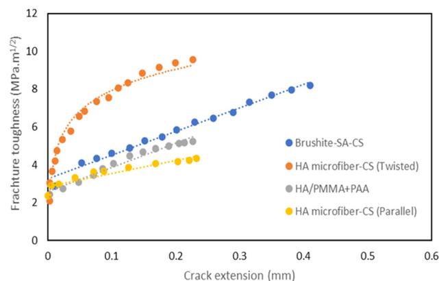
Fig. 16 Rising R-curves for the selected composites. Data points extracted from.<sup>78,81,84,88</sup>
