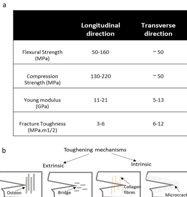
**Fig. 2** (a) The mechanical properties of cortical bone. It shows the anisotropy behavior of materials. (b) Toughening mechanisms of bone: illustration depicting the structural features and intrinsic and extrinsic mechanisms that contribute to the remarkable toughness of bone tissue.<sup>23–25</sup>
