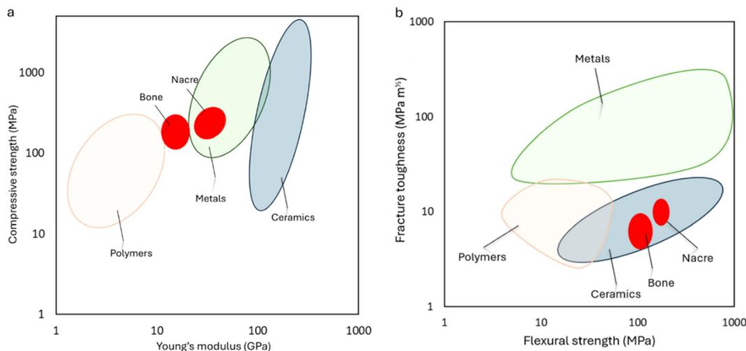
**Fig. 5** Exploring material strength: Ashby plot contrasts the mechanical properties of diverse materials with those of bone and nacre, offering insights into the relative performance and suitability for various engineering applications. (a) Compressive strength based on Young's modulus, (b) fracture toughness is based on Flexural strength. The data extracted from ref. 27, 29, 64–69.
