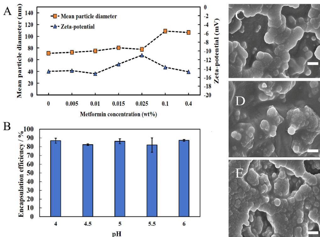
**Fig. 2** (A) The mean particle diameter and zeta-potential of Ly-NPs at different metformin payloads. (B) The encapsulation efficiency of Ly-NPs at different pH levels. (C) SEM image of 0.2 wt% shellac–0.25 wt% lysozyme–0.1 wt% metformin–0.25 wt% P407 NPs. (D) SEM image of 0.2 wt% shellac–0.25 wt% lysozyme–0.2 wt% metformin–0.25 wt% P407 NPs. (E) SEM image of 0.2 wt% shellac–0.25 wt% lysozyme–0.4 wt% metformin–0.25 wt% P407 NPs. The scale bar is 100 nm.
