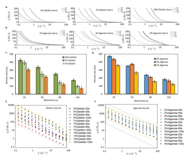
Fig. 2 FRESH-specific rheological response of different slurries made of (A) 5, 7, and 10% w/v gelatin and (B) 2, 3, and 4% w/v agarose, utilizing 20, 50, 80, and 120 s blend time; the average microparticle size obtained after blending the (C) gelatin and (D) agarose slurries; the calculated master curve locus obtained for (E) gelatin and (F) agarose slurries.
