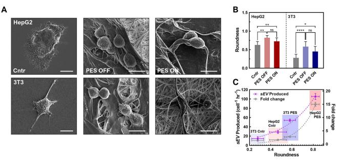
Fig. 5 (A) SEM images of HepG2 and 3T3 fibroblast cells under three different cultures including 2D, PES OFF, and PES ON cultures (scale bar: 10 µm). (B) The cell measurement through roundness. (C) The correlation between the roundness and the sEV production rate and fold change in production rate post stimulation. All data shown as  $\pm$ S.D. of 3 replicate samples is representative of two independent experiments: \*P < 0.05, \*\*P < 0.01\*\*\*P < 0.001, and \*\*\*\*P < 0.0001.
