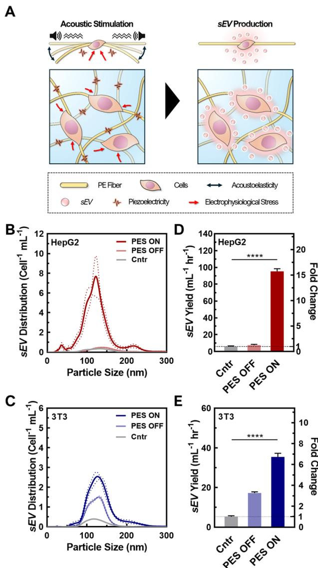
**Fig. 2** (A) Schematic of the piezoelectric stimulation that enhances sEV production. (B and C) Size distribution of sEVs derived from (B) HepG2 and (C) 3T3 cells using NTA. Data shown as  $\pm$ S.D. of 5 replicate samples. (D and E) Measured sEV production rate per cell from (B) HepG2 and (C) 3T3 using ExoELISA. Data shown as  $\pm$ S.D. of 5 replicate samples: \*\*\*\* $P < 0.0001$ .
