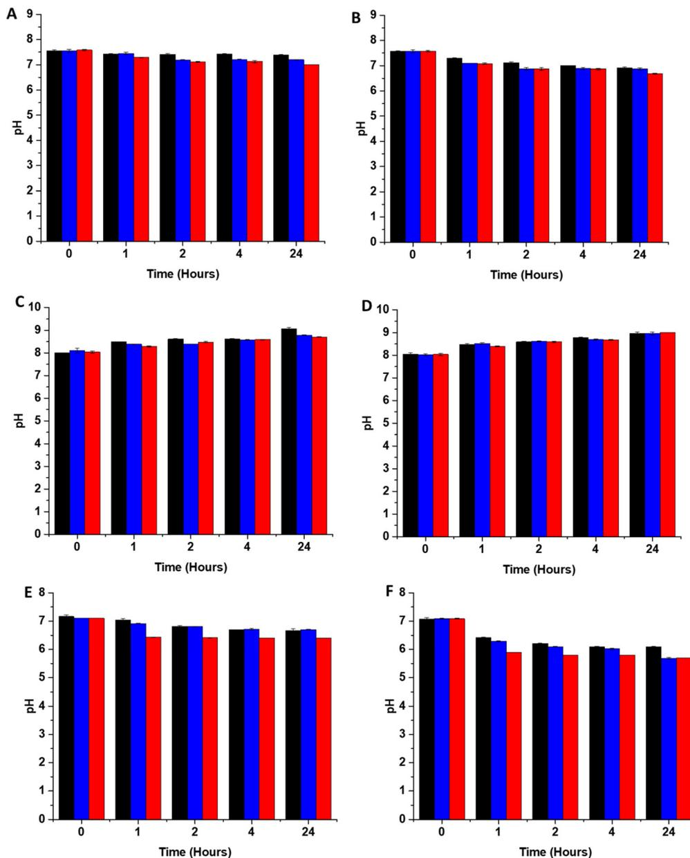
**Fig. 4** pH changes of solutions containing SNAP coated substrates at room temperature (RT) and at 37 °C (A) PBS RT (B) PBS 37 °C (C) DMEM RT (D) DMEM 37 °C (E) LB broth RT (F) LB broth 37 °C. Black 2 w/v%; blue 4 w/v%/OC; red 4 w/v%. The pH change observed upon release of  $\text{HNO}_2$  is dependent on the amount of immobilised SNAP and the buffering capacity of the solution. Values represent mean  $\pm$  SD ( $n = 3$ ).
