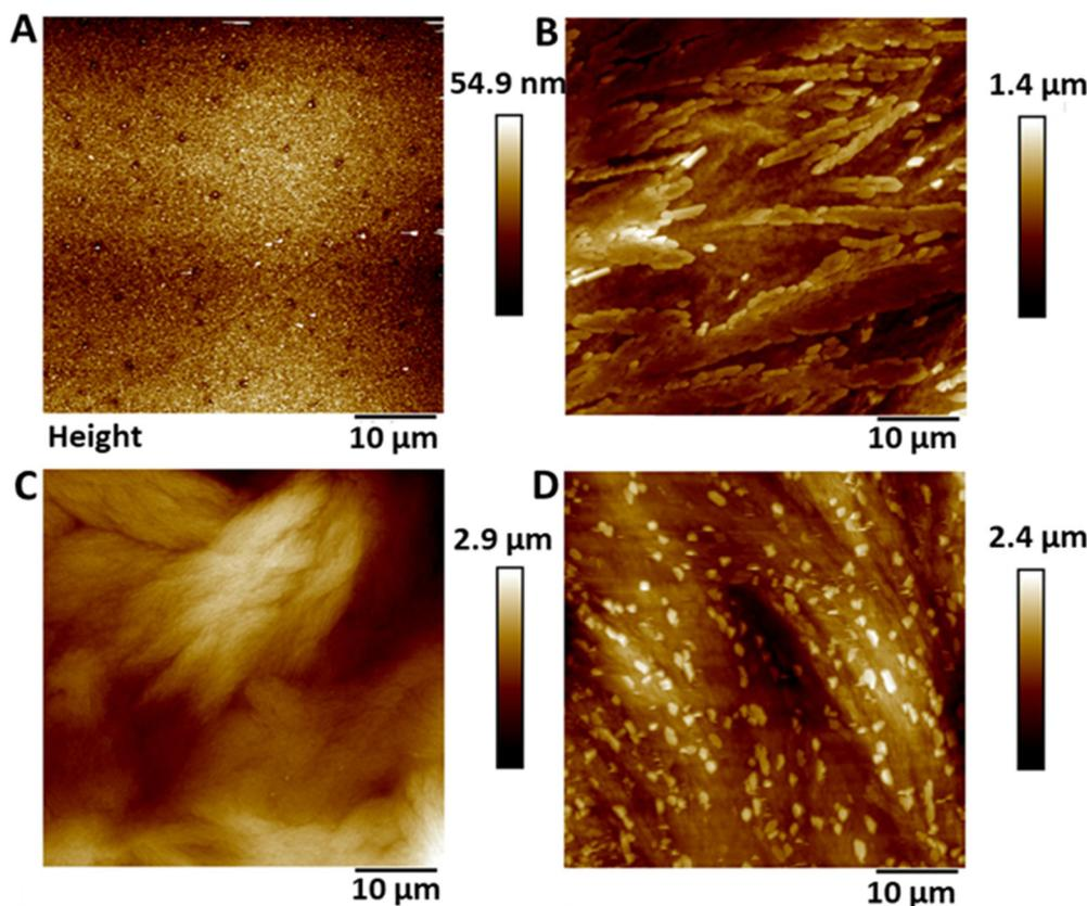
**Fig. 1** Representative AFM height profiles of (A) Control Elast-Eon (B) 2 w/v% (C) 4 w/v% and (D) 4 w/v% OC. As the concentration of SNAP in the coating is increased, the surface height/topography increases.
