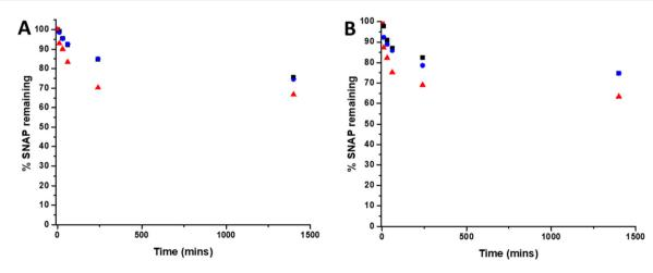
Fig. 3 Graphs showing % SNAP remaining in SNAP coated substrates at (A) room temperature (RT) and (B) 37 °C. Black 2 w/v%; blue 4 w/v%/OC; red 4 w/v%. Values represent mean  $\pm$  SD (n = 3).
