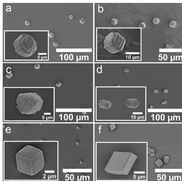
**Fig. 4** SEM micrographs of crystals obtained using the ADM method in the presence of (a) ABA-1, (b) ABA-2, (c) CBA-1, (d) CBA-2, (e) the control Affimer protein, and (f) in the absence of any protein.
