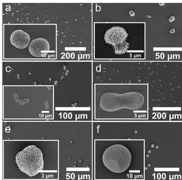
**Fig. 5** SEM micrographs of crystals obtained using the ADM method in the presence of  $\text{Mg}^{2+}$  ions at a Ca:Mg ratio 1:1 and (a) ABA-1, (b) ABA-2, (c) CBA-1, (d) CBA-2, (e) the control Affimer protein, and (f) in the absence of any protein. The images shown in the insets are (a and b) aragonite crystals and (c–f) calcite crystals.
