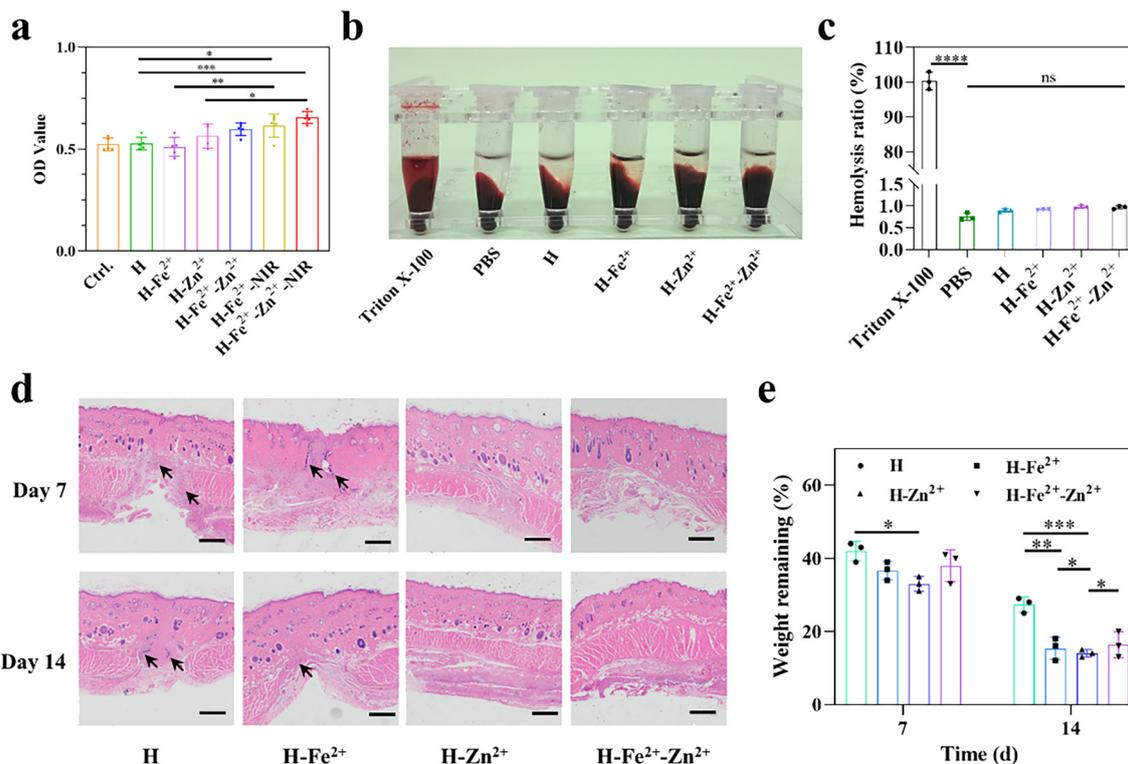
**Fig. 2** Biocompatibility evaluation of the PGA composite hydrogels. (a) The proliferation activity of L929 cells; (b) representative digital photos of hemolysis experiments; (c) hemolysis ratio; (d) representative H&E staining images of the skins near subcutaneous implantation (scale bar = 500  $\mu$ m; the black arrow points towards inflammatory cells); and (e) weight remaining *in vivo* ( $n = 3$ ,  $*p < 0.05$ ,  $**p < 0.01$ ,  $***p < 0.001$ ,  $****p < 0.0001$ ).
