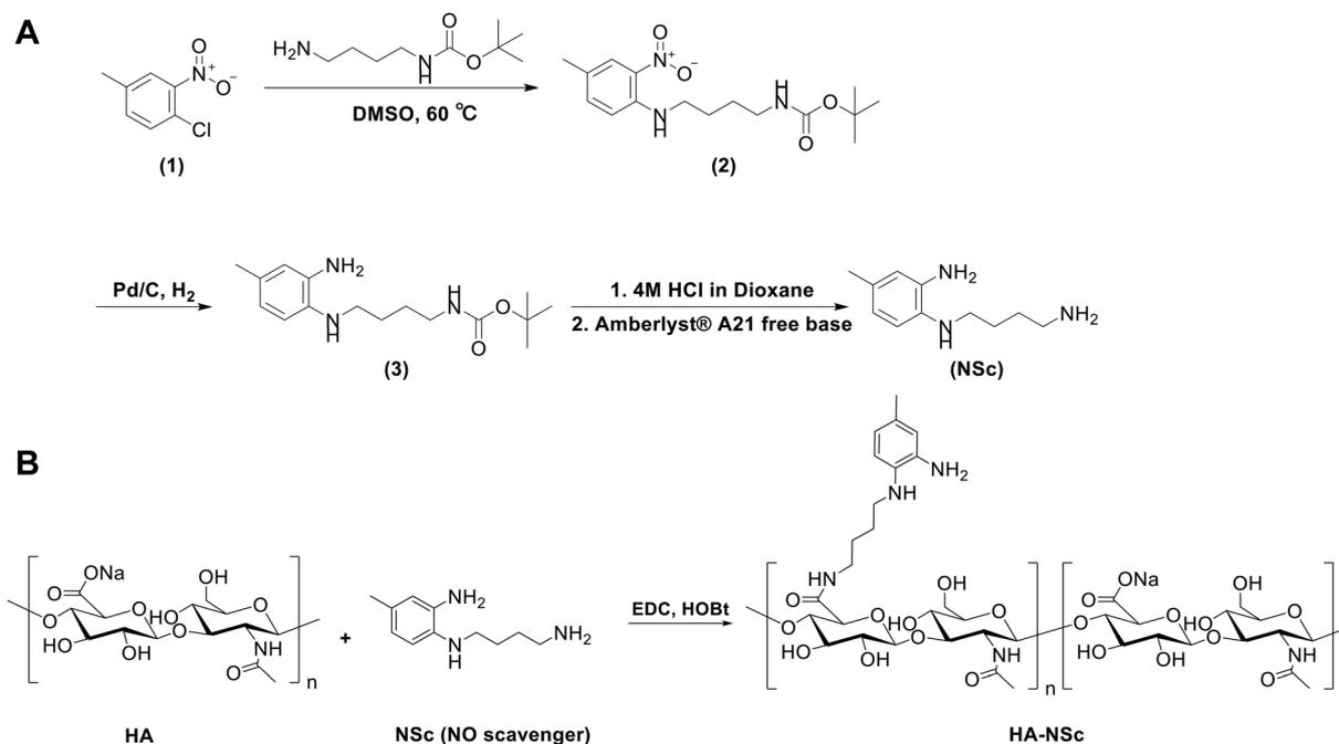
Fig. 1 (A) Synthesis of *N*<sup>1</sup>-(4-aminobutyl)-5-methylbenzene-1,2-diamine (NSc). (B) Synthesis of HA-NSc conjugate.
