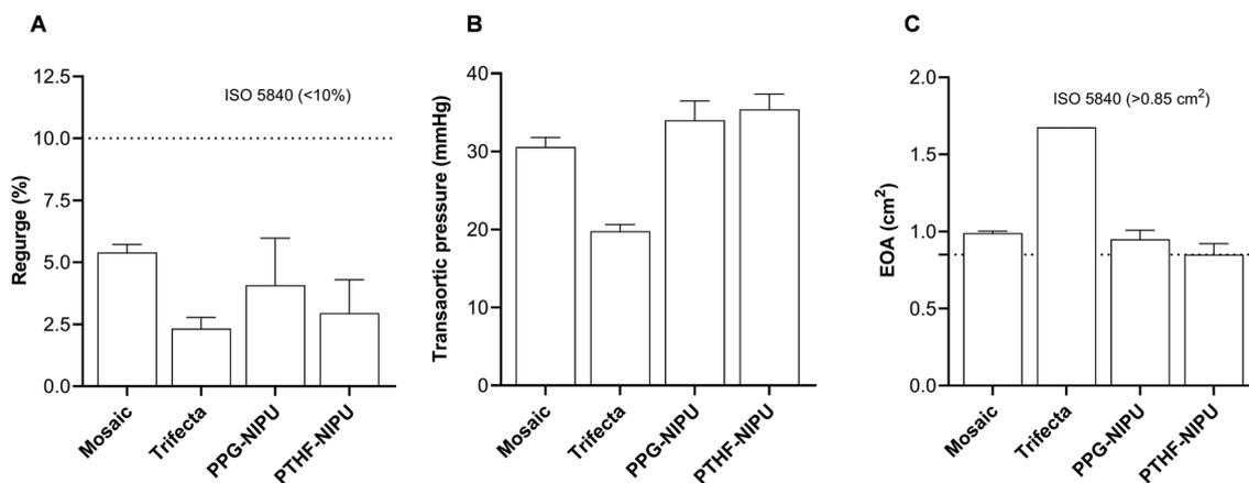
**Fig. 6** Hydrodynamic parameters of *Mosaic* and *Trifecta* bioprostheses, PPG-NIPU and PTHF-NIPU valves. (A) Regurgitation fraction; (B) transaortic pressure; (C) effective orifice area (EOA). Parameters were measured in a pulse duplicator with normotensive conditions. Data are presented as mean with SD ( $n = 2-6$ ).
