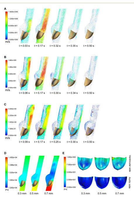
Fig. 3 Velocity vectors, transvalvular pressure gradient and shear stress magnitude for different leaflet thicknesses. Velocity vectors (m s<sup>-1</sup>) of blood flow at different time points in the cardiac cycle through 0.3 mm (A), 0.5 mm (B) and 0.7 mm (C) leaflets; (D) pressures at peak systole for the 0.3 mm, 0.5 mm and 0.7 mm leaflets; (E) shear stresses and streamlines on the ventricular and aortic sides at peak systole for the 0.3 mm, 0.5 mm and 0.7 mm leaflets.
