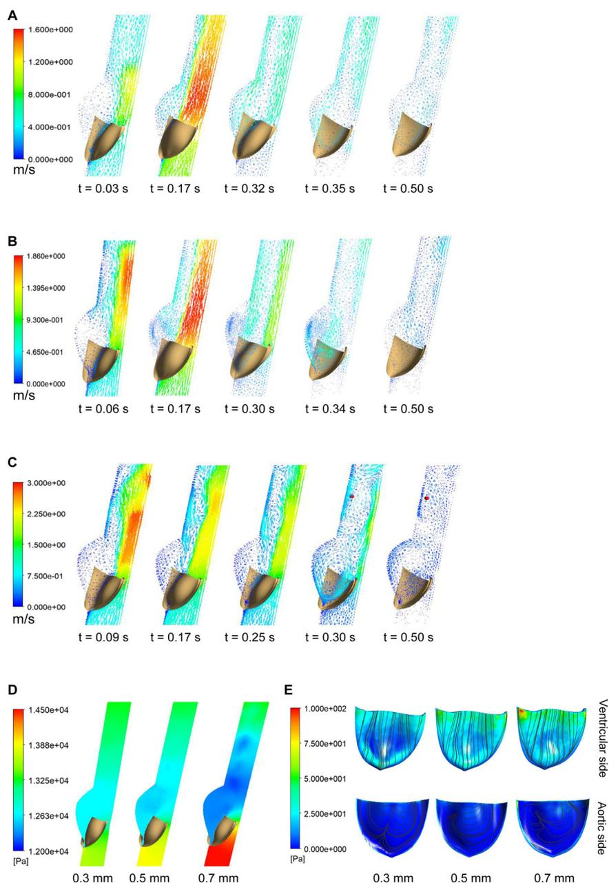
**Fig. 3** Velocity vectors, transvalvular pressure gradient and shear stress magnitude for different leaflet thicknesses. Velocity vectors ( $\text{m s}^{-1}$ ) of blood flow at different time points in the cardiac cycle through 0.3 mm (A), 0.5 mm (B) and 0.7 mm (C) leaflets; (D) pressures at peak systole for the 0.3 mm, 0.5 mm and 0.7 mm leaflets; (E) shear stresses and streamlines on the ventricular and aortic sides at peak systole for the 0.3 mm, 0.5 mm and 0.7 mm leaflets.
