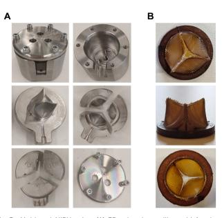
Fig. 5 Mold and NIPU valve. (A) 3D-printed metallic mold (made of stainless steel 316L) and its different parts; (B) top, side and bottom views of a 19 mm (internal diameter) valve produced by injection molding. The insertion of a metallic stent can be observed, as well as the outer support ring.
