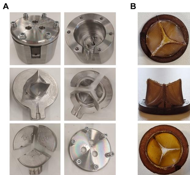
**Fig. 5** Mold and NIPU valve. (A) 3D-printed metallic mold (made of stainless steel 316L) and its different parts; (B) top, side and bottom views of a 19 mm (internal diameter) valve produced by injection molding. The insertion of a metallic stent can be observed, as well as the outer support ring.
