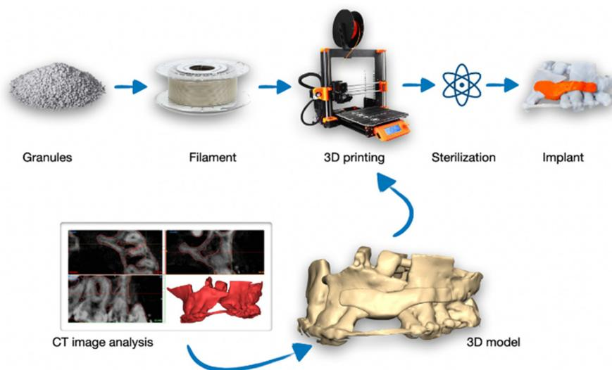
Fig. 7 General diagram of the *Cranioimplant* manufacturing process.
