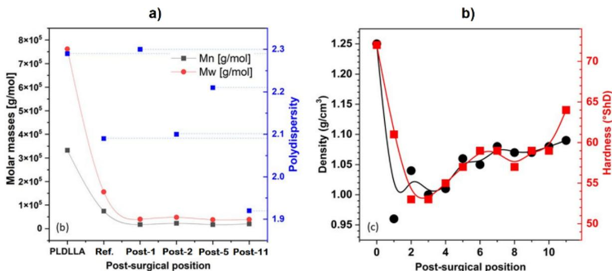
Fig. 4 (a) Number-average molar mass ( $M_n$ ), weight-average molar mass ( $M_w$ ) and polydispersity ( $D$ ) of the as-received PLDLLA, the processed polymer (after melt mixing and 3D printing – Ref) and of the grafted material, with representative samples taken at the indicated sites (post-surgical samples); (b) density (black circles) and hardness (red squares) values for the reference nHAp@PLDLLA and post-surgical samples, reported as function of position within the implant.
