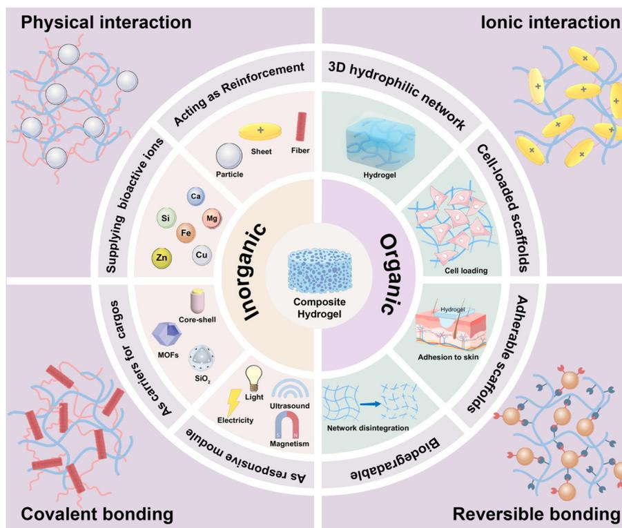
**Scheme 1** Schematic diagram showing the interaction and functionalization of two constituent components within organic–inorganic composite hydrogels that they exhibit a diverse range of interactions and modulations on hydrogel performances from respective aspects.
