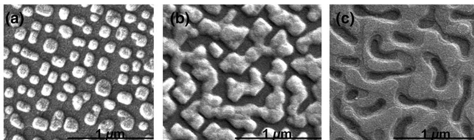
**Fig. 3** Scanning electron microscopy of the patterns (nanofeatures) obtained from selectively chemically etching bioactive glass solid disks and porous scaffolds manufactured using the GDC/YSZ system: (a) islands, (b) connected islands, and (c) pits. Scale bar of each micrograph equal to 1  $\mu\text{m}$ . Reprinted from ref. 318 (Copyright © 2012) with permission from Elsevier.
