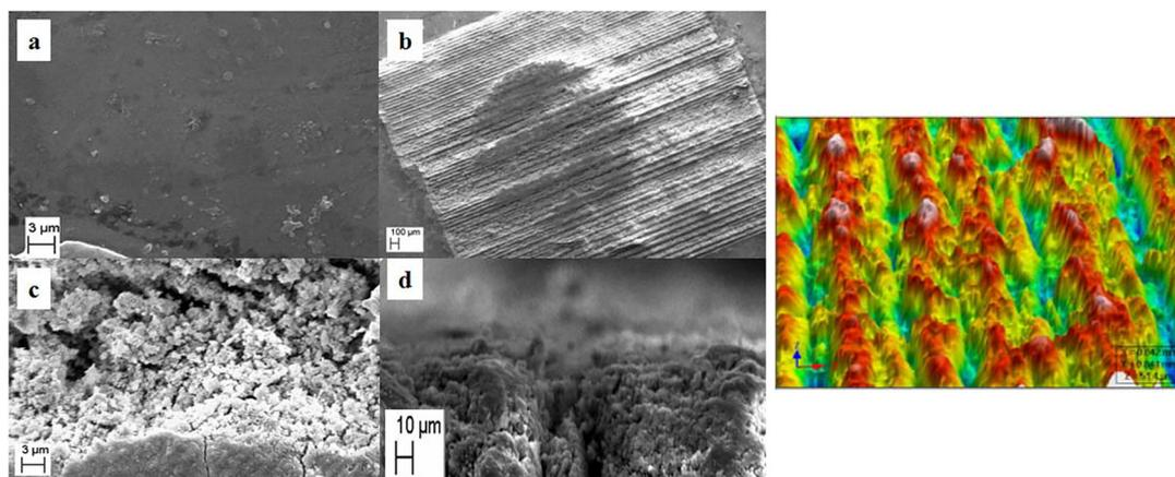
**Fig. 2** 45S5 Bioglass® samples treated with femtolaser, reproduced from ref. 342 with permission of the Laser Institute of America: left – SEM images of (a) the surface of untreated BG, (b, c) laser-treated region of BG at low (46X) and high (3KX) magnification and (d) cross-sectional view of laser-treated BG, with scale bars of  $3 \mu\text{m}$ ,  $100 \mu\text{m}$ ,  $3 \mu\text{m}$  and  $10 \mu\text{m}$ , respectively; right – 3D optical image of laser-treated BG.
