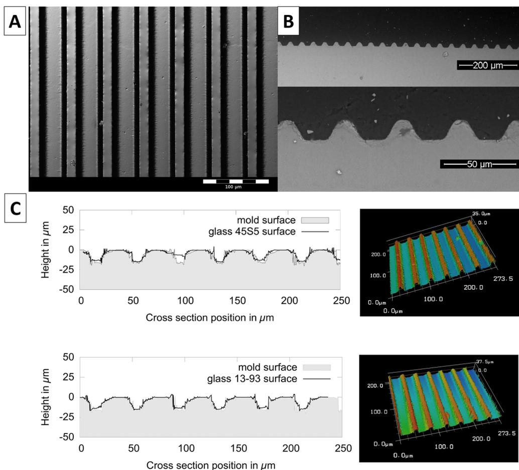
**Fig. 4** Microstructured 45S5 Bioglass® and 13-93<sup>358</sup> with permission of DeGruyter: (A) surface of glass 13-93; (B) SEM micrographs of the cross-section of cast bioactive glass 45S5 showing the surface microstructure; (C) 2D laser scanning profile of the surface microstructure on bioactive glass 45S5 (top) and 13-93 (bottom) superimposed with a 2D scan of the mold surface, as well as 3D laser-scanning profiles of the glass surfaces of 45S5 and 13-93 (right).
