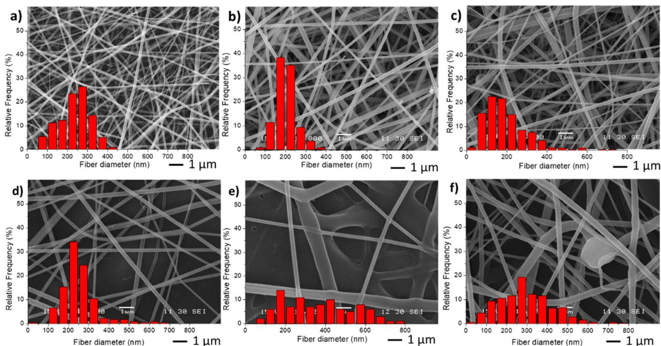
**Fig. 3** SEM images and diameter distribution from fiber samples M0 (a), M1(b), M2 (c), M3 (d), M4 (e) and M5 (f).
