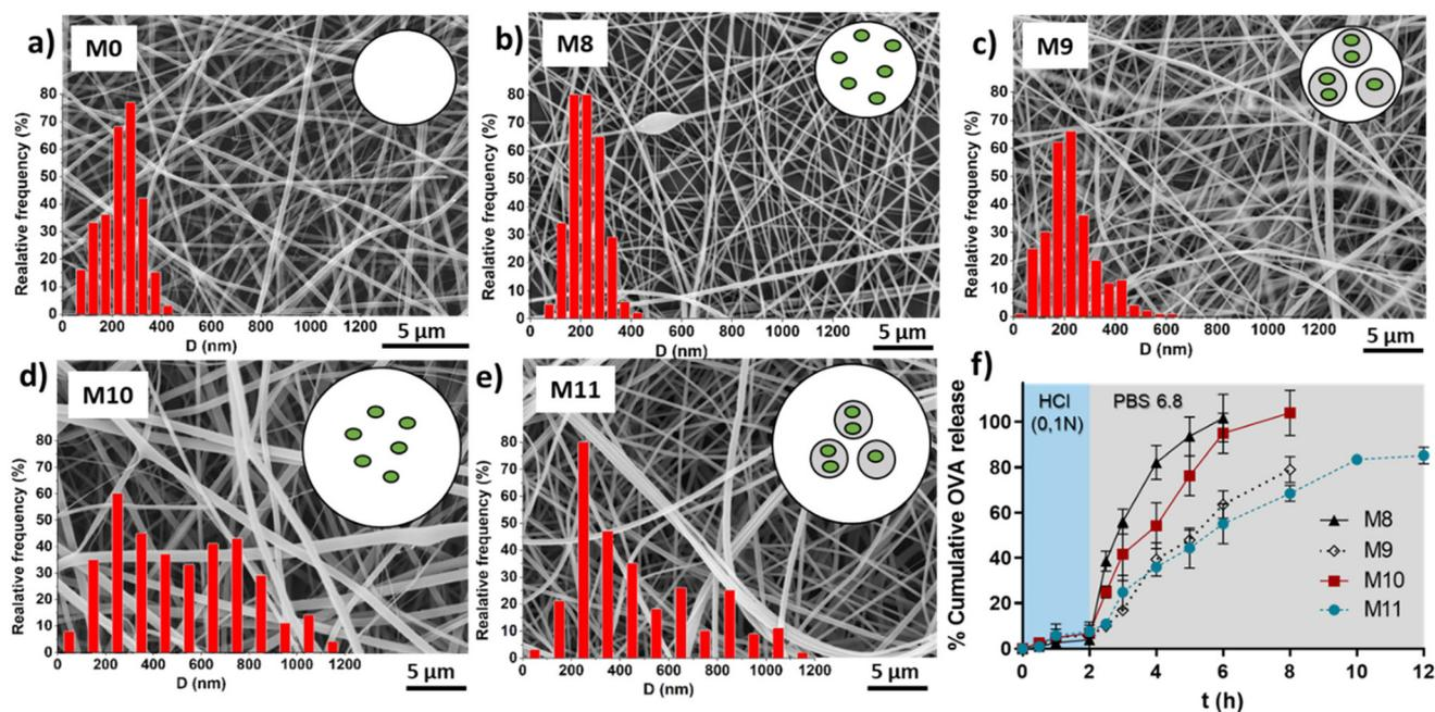
**Fig. 8** SEM images and scheme of a transversal cut of fibers M0 (a), M8 (b), M9 (c), M10 (d) and M11 (e). OVA release from M8, M9, M10 and M11 incubated for 2 h in HCl 0.1 N and then in PBS pH 6.8 until complete fibers dissolution (f).
