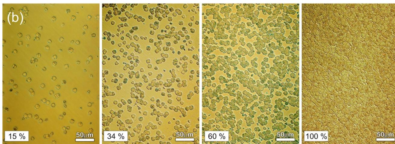
**Fig. 5** Effect of crystallization percentage on mechanical properties of a phospho-silicate combeite glass-ceramic. (a) Flexural strength vs. fraction crystallized during a multistage heat treatment schedule. (b) Optical microscope images showing microstructure examples of increasingly crystallized glass-ceramic samples. From ref. 112 with permission from Elsevier, 2001.
