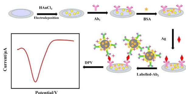
**A sandwich electrochemical immunosensor based on polypyrrole microspheres for the detection of the cancer marker CA125**
