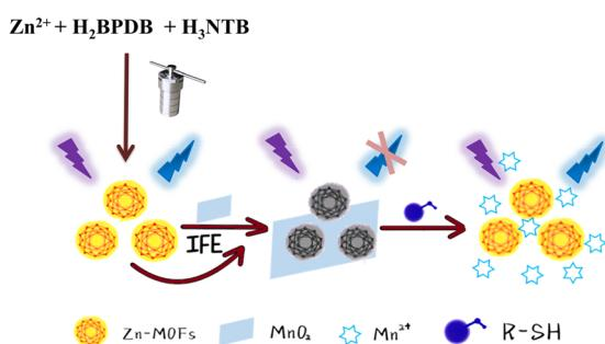
**Synthesis of a Zn-MOF fluorescent material for sensitive detection of biothiols via an inner filter effect with  $MnO_2$  nanosheets**
