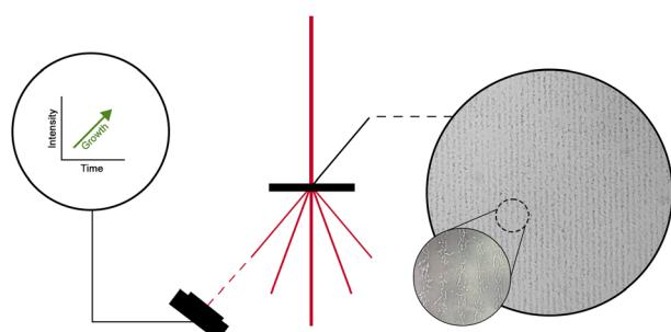
**Low-cost, real-time detection of bacterial growth via diffraction-based sensing**
