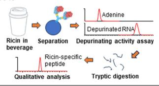
Simultaneous analysis of depurinated nucleic acid stem-loop and free adenine for ricin toxicity assay by hydrophilic interaction liquid chromatography-highresolution mass spectrometry (HILIC-HRMS)
