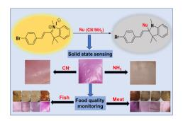
An indolium ion-based colorimetric sensor for naked-eye detection of cyanide and ammonia: on-site detection technique for cyanide in natural sources and day-to-day monitoring of food spoilage
